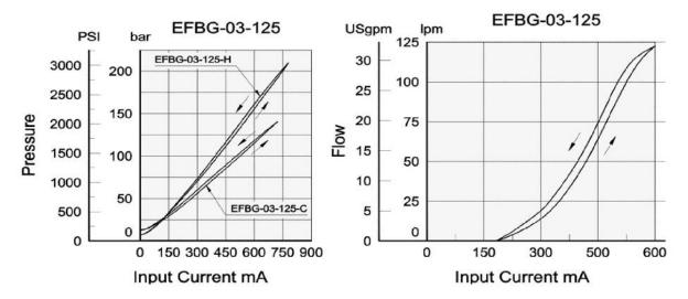
EFBG-03 Proportional Electro-Hydraulic Relief and Flow Control Valves (10Ω-10Ω Series)
